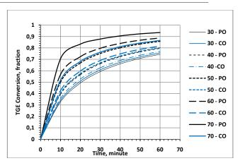
Fig.5: The Calculated Palm and Coconut Oil TGE conversion base on a second order of pseudo homogeen reaction with parameters of the reaction temperature and the reaction duration time.
