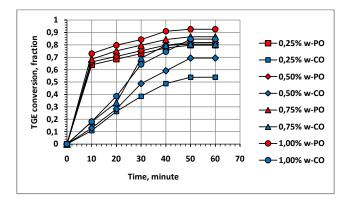
Fig.3: The effect of catalyst and time duration on the Palm and Coconut TGE conversion with the reation temperature of 70 °C , the MET/TGE ratio of 5, NaOH catalyst of 1% and ultrasonic activation of 30 minutes.
