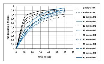
Fig.9: The Calculated Palm and Coconut Oil TGE conversion base on a second order of pseudo homogeen reaction with parameters of the ultrasonic catalyst activation and the reaction duration time.
