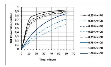
Fig.7: The Calculated Palm and Coconut Oil TGE conversion base on a second order of pseudo homogeen reaction with parameters of the NaOH catalyst amount and the reaction duration time.
