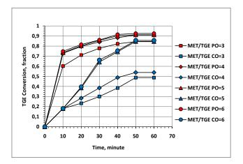
Fig.2: The effect of the MET/TGE ratio and time duration on the Palm and Coconut TGE conversion with the reation temperature of 70 °C, NaOH catalyst of 1% and ultrasonic activation of 30 minutes.
